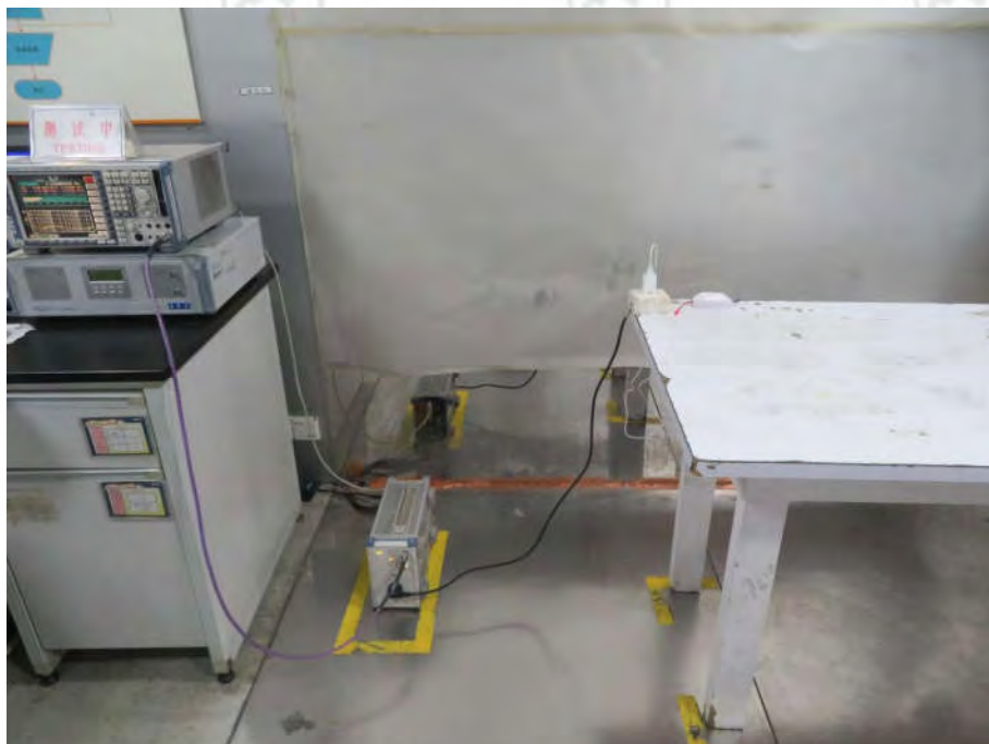
Conducted Emissions Test Setup
