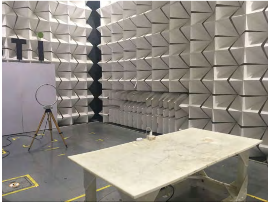
Radiated spurious emission Test Setup-1(Below 30MHz)
