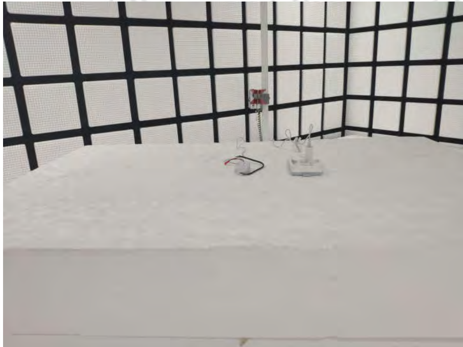
Radiated spurious emission Test Setup-3(Above 1GHz)
