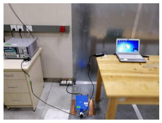
FCC RADIATED EMISSION TEST SETUP BELOW 1GHZ
