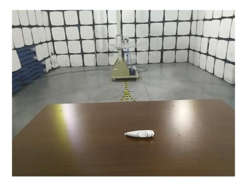
Radiation Emission Test Setup (1GHz to 18GHz)
