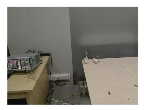
Radiation Emission Test Setup (Below 30MHz)
