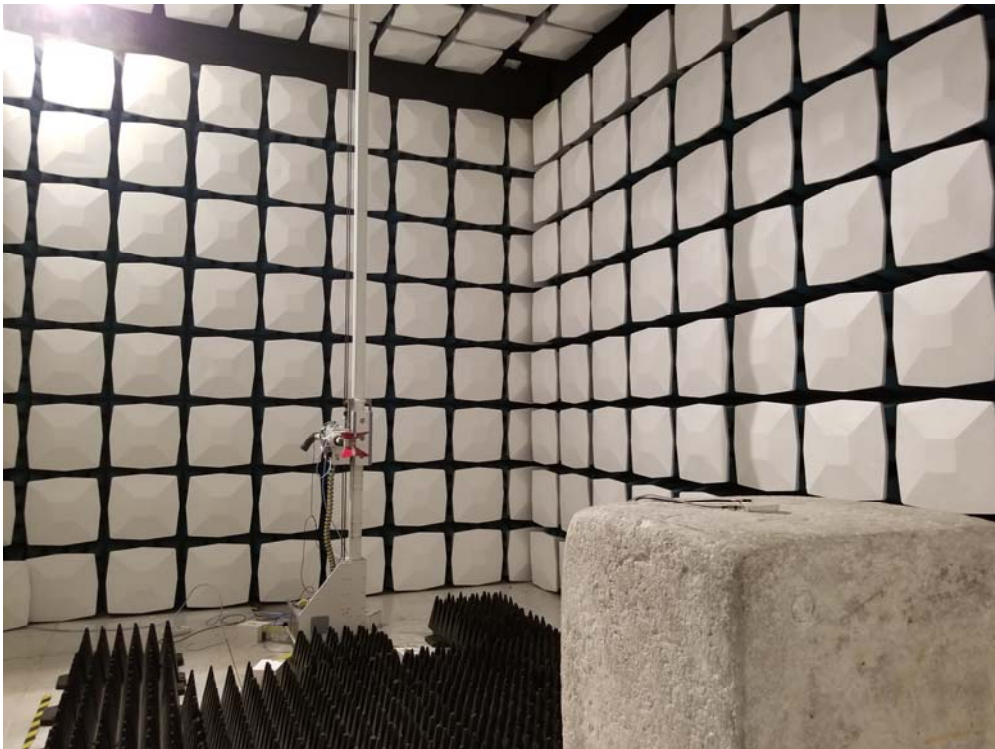
Description: Radiated Emission Test Setup for 1~18GHz
