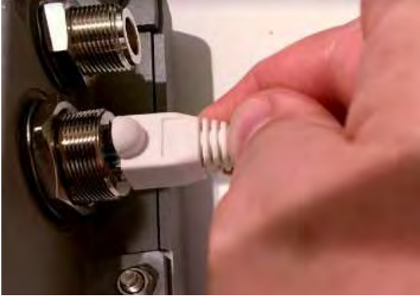
Figure 6: Connecting the Ethernet cable to the gateway
