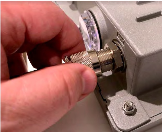
Figure 5: Connecting the LoRa antenna to the gateway
