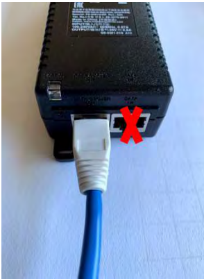
Figure 7: Ethernet cable connected to the power brick
