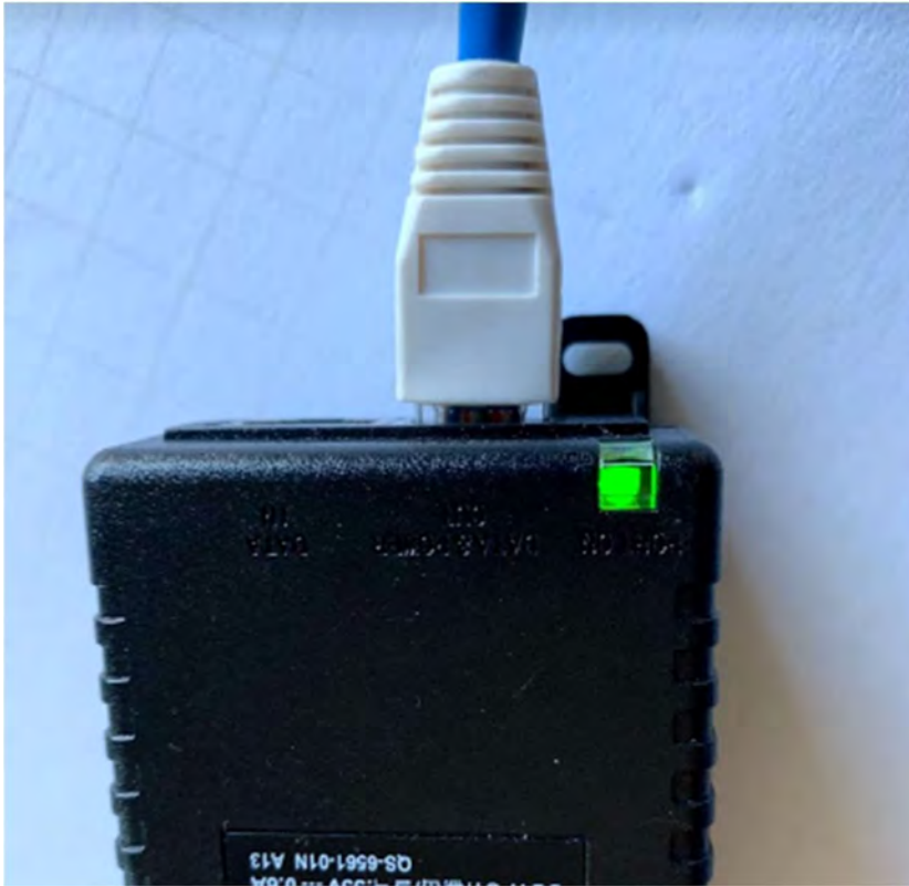
Figure 12: Green LED on Power Brick Means Gateway is Powered
