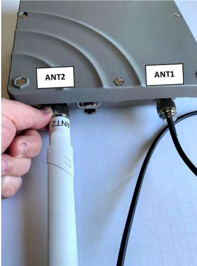
Figure 8: Connecting the Cellular antenna to the gateway
