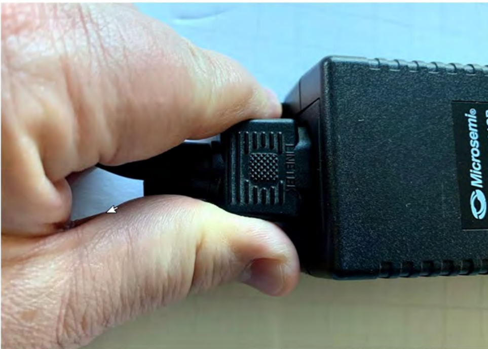
Figure 11: Connecting mains cable to power brick
