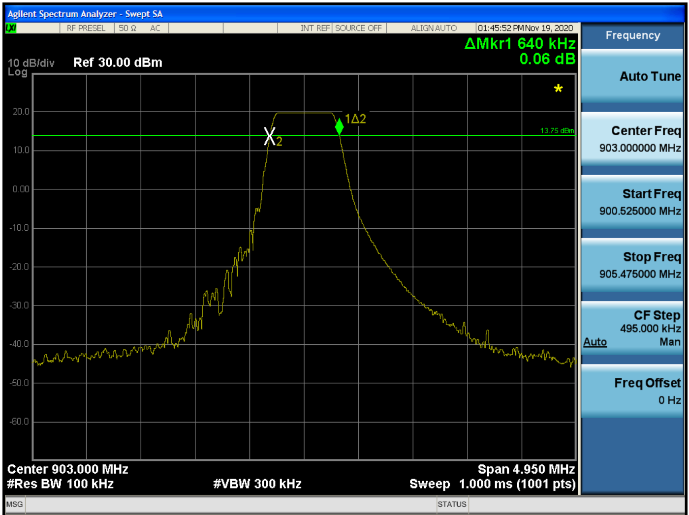
DTS Bandwidth – Low Channel
