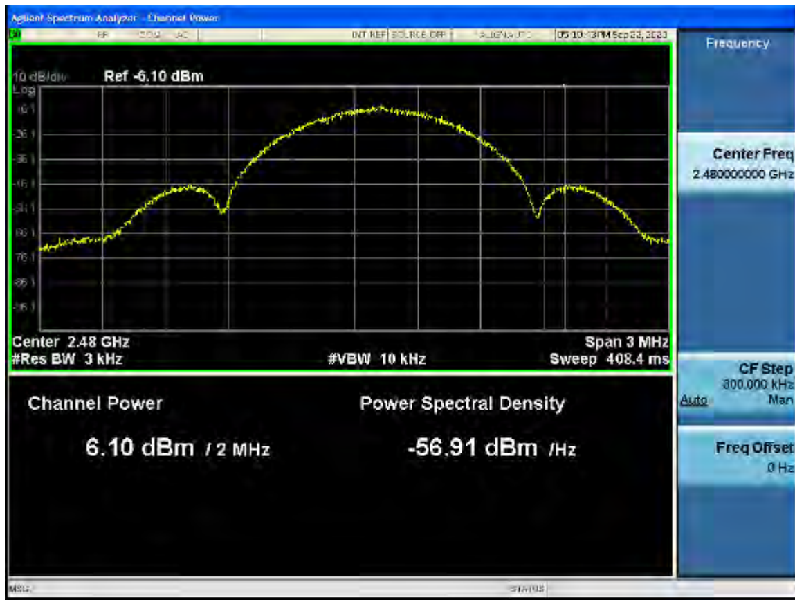
Power Spectral Density – High Channel
