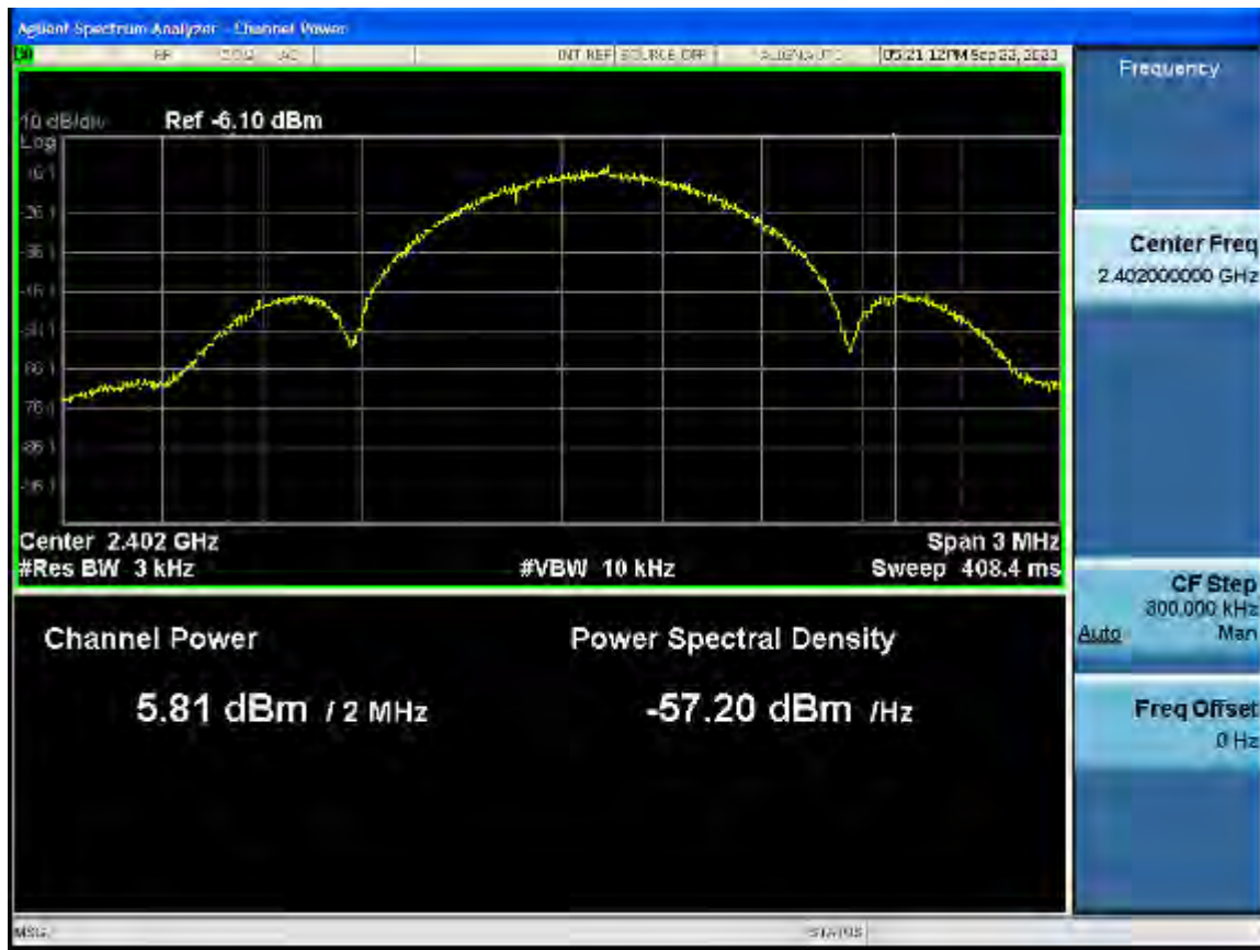
Power Spectral Density – Low Channel
