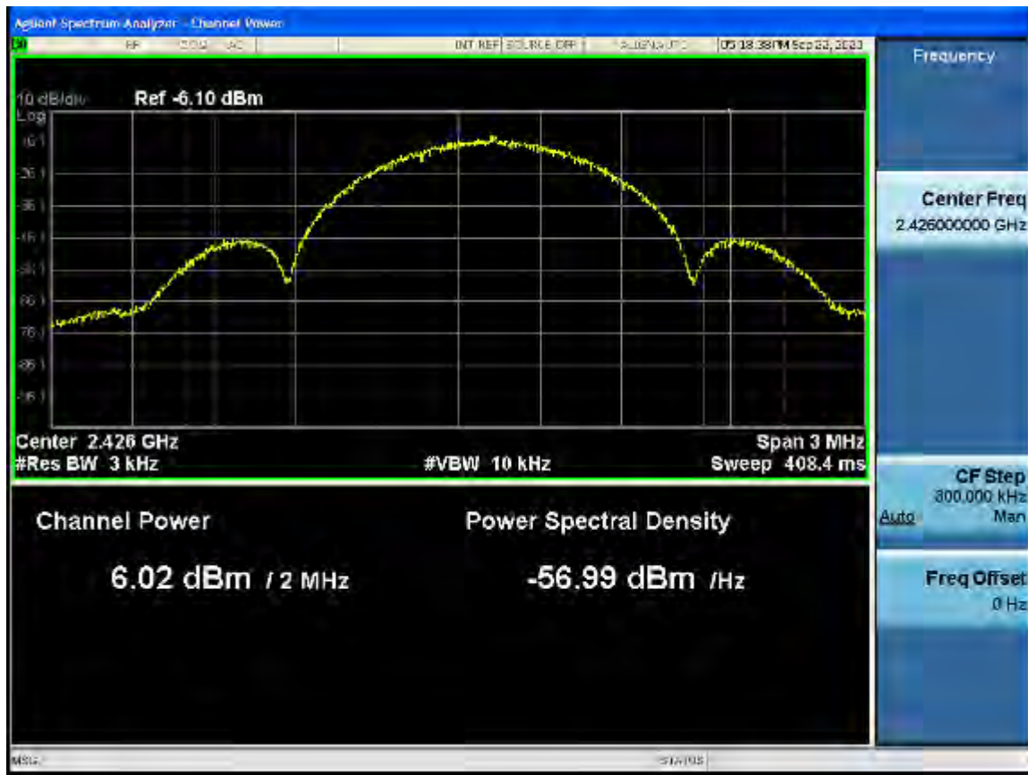
Power Spectral Density – Middle Channel
