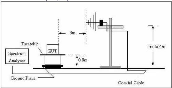
(C) Radiated Emission Test-Up Frequency Above 1GHz
