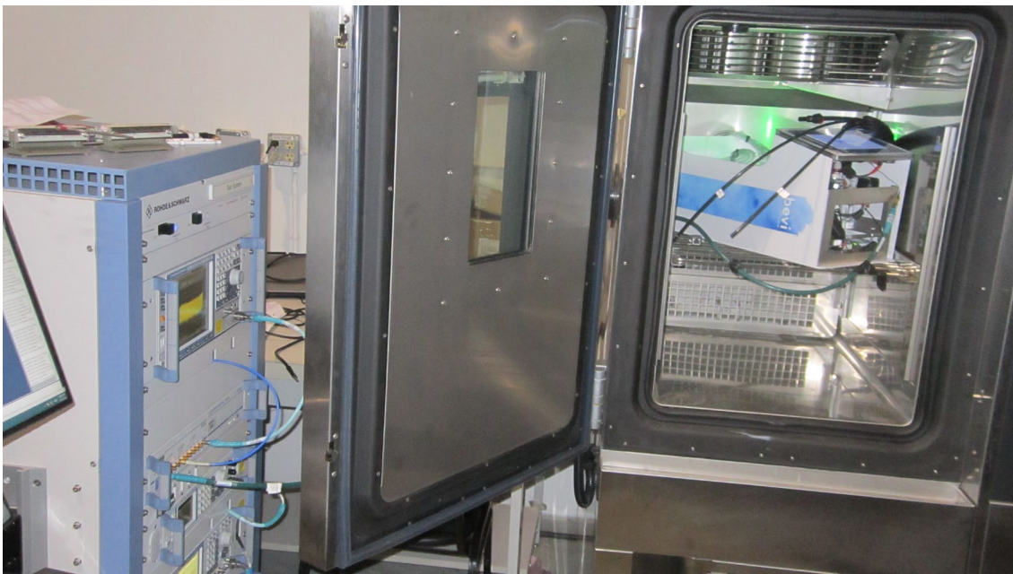
Frequency stability setup, 1
