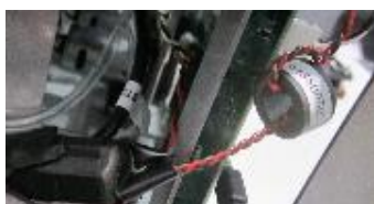
Power Cable from Control Board to SOM one Ferrite with one loop near control board PN 2643800502 and one ferrite right next to it PN 0461167281
