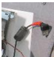
USB Cable near 90 degree Connector Ferrite PN 0444164281
