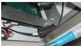
One Ferrite on LED Cable PN: 0431164281
