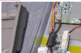
One Ferrite on the LVSD Cable under the Plastic Cover PN 0461178181
