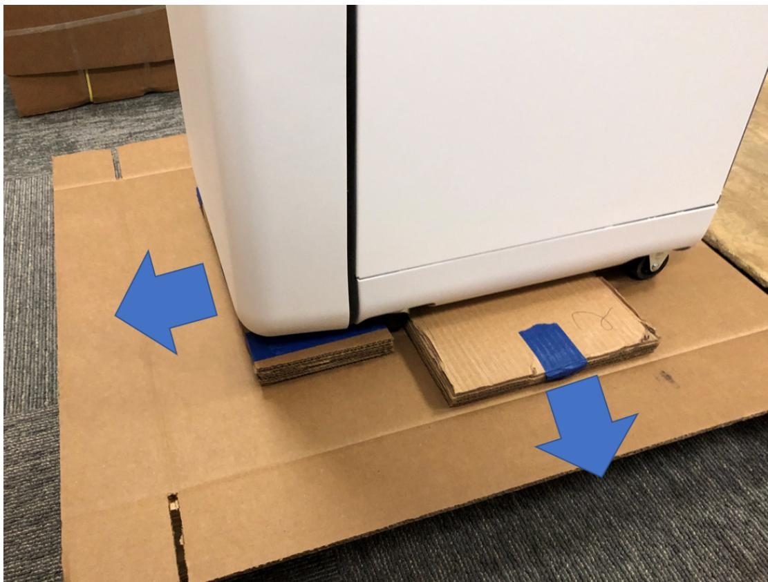
3. Roll the machine toward the front edge of the pallet to allow space behind the rear of the machine.
