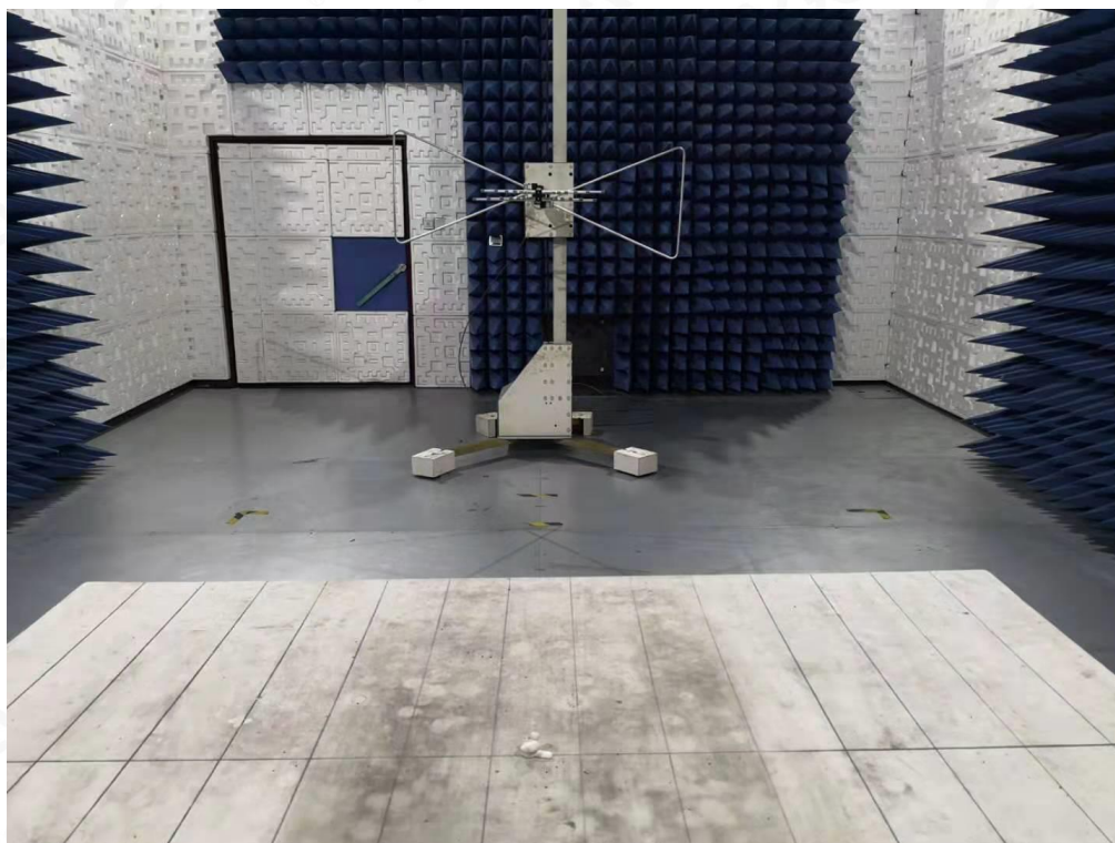
RADIATED EMISSION TEST SETUP ABOVE 1GHZ
