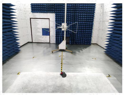
RADIATED EMISSION TEST SETUP ABOVE 1GHz
