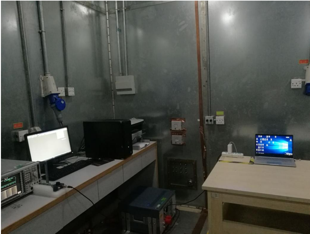
FCC RADIATED EMISSION TEST SETUP BELOW 1GHZ
