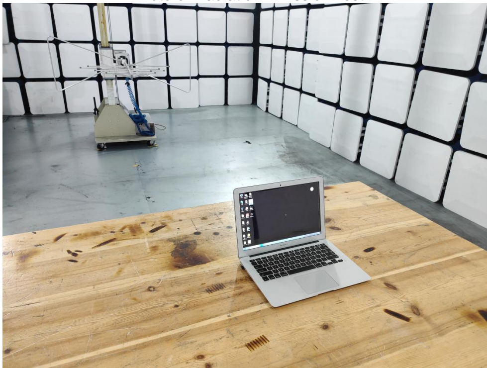
Photo of Radiation Emission Test
