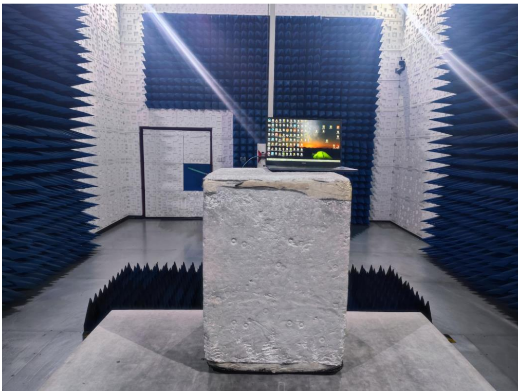
RADIATED EMISSION TEST SETUP ABOVE 1GHZ
