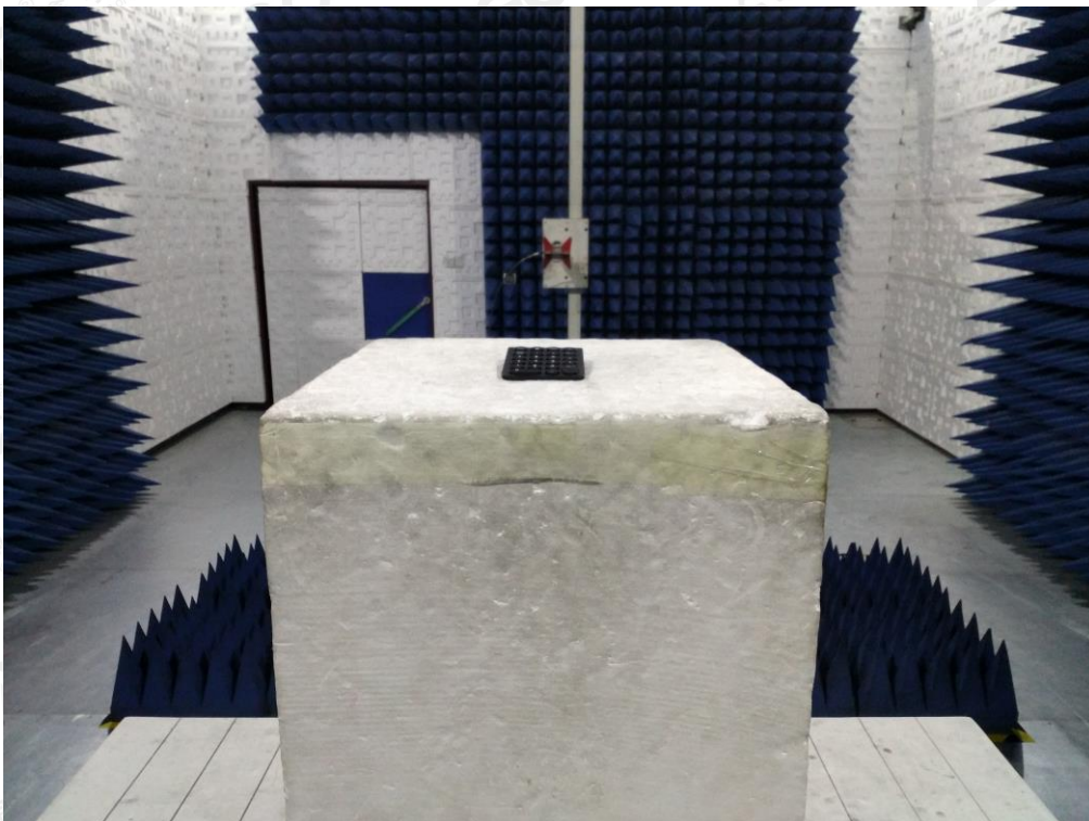
RADIATED EMISSION TEST SETUP ABOVE 1GHZ
