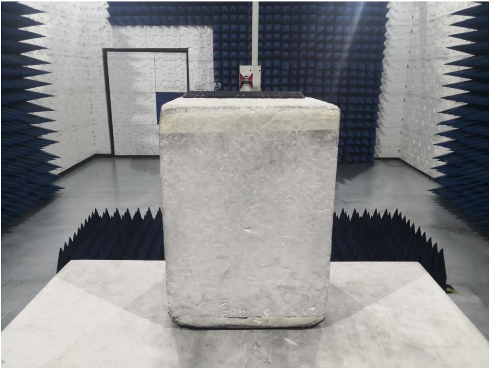
RADIATED EMISSION TEST SETUP ABOVE 1GHz
