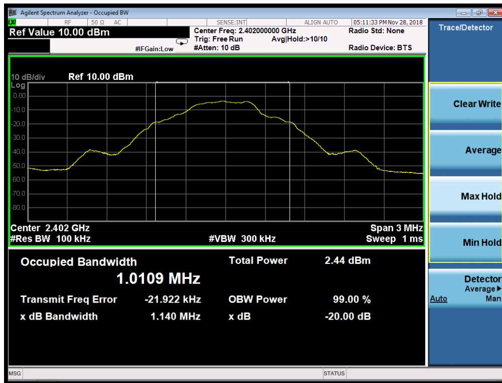
TEST PLOT OF BANDWIDTH FOR LOW CHANNEL
