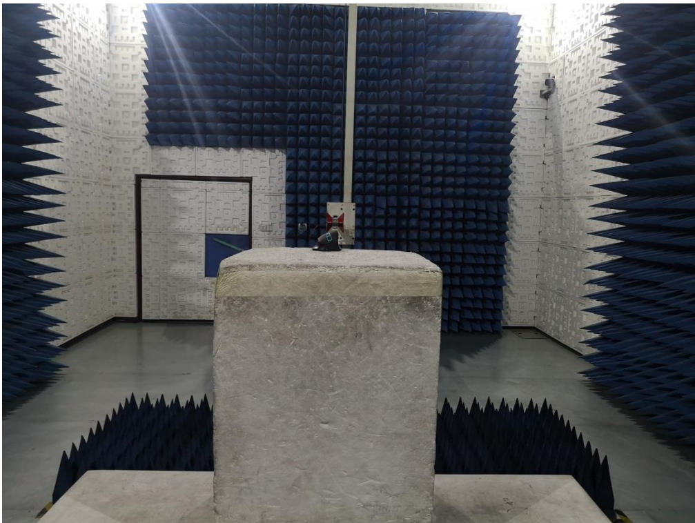
RADIATED EMISSION TEST SETUP ABOVE 1GHZ
