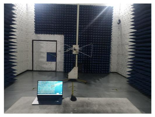
RADIATED EMISSION TEST SETUP ABOVE 1GHZ
