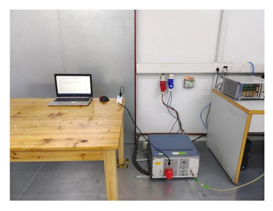
CONDUCTED TEST SETUP
