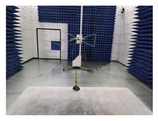
RADIATED EMISSION TEST SETUP ABOVE 1GHz
