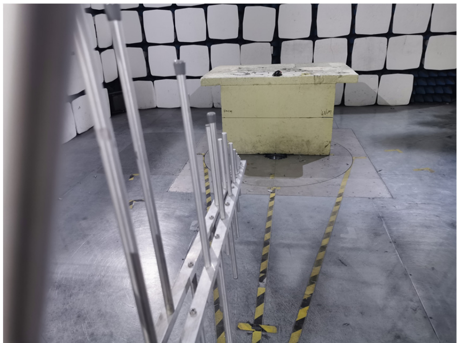
Radiation Emission Test Setup (30MHz to 1GHz)
