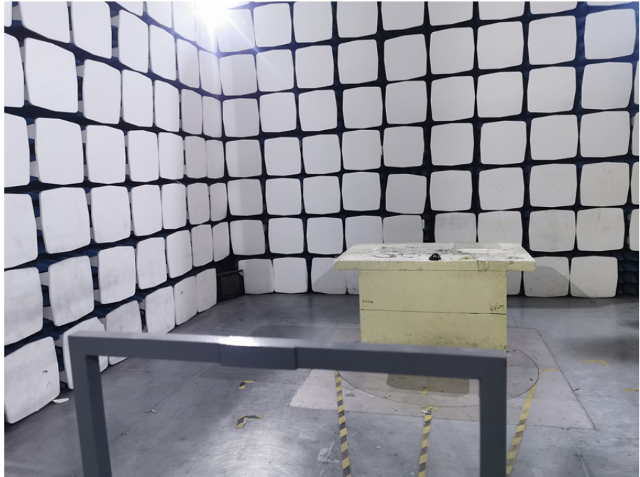
Radiation Emission Test Setup (Below 30MHz)
