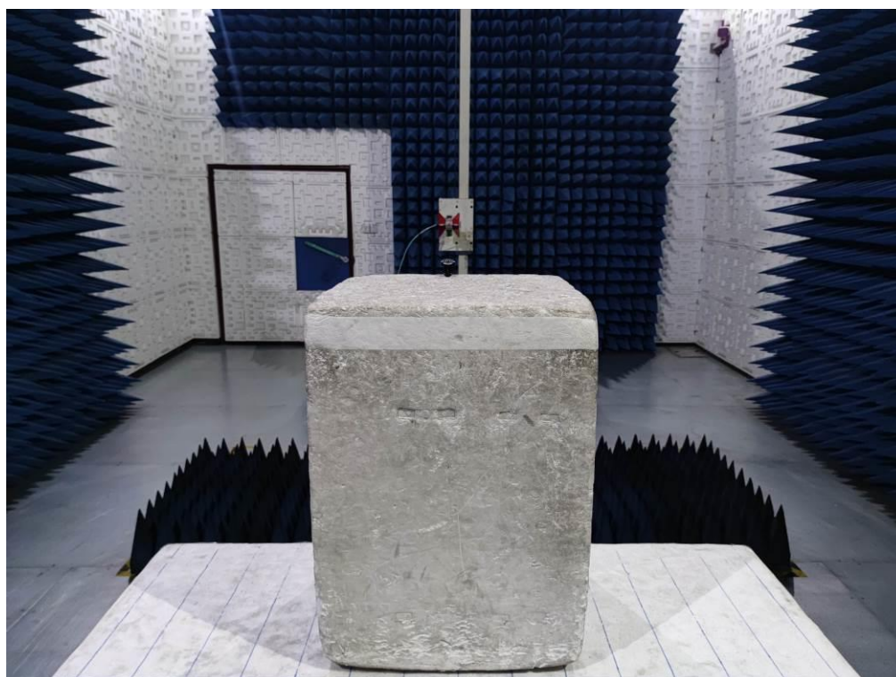
RADIATED EMISSION TEST SETUP ABOVE 1GHz
