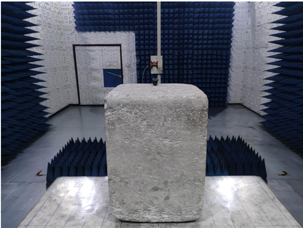
RADIATED EMISSION TEST SETUP ABOVE 1GHz
