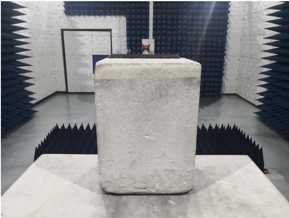
RADIATED EMISSION TEST SETUP ABOVE 1GHZ
