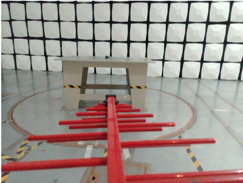
Radiated Emission Below 1GHz front View
