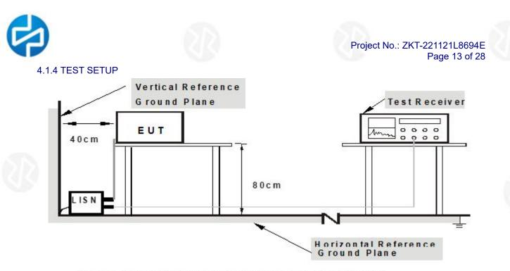
Note: 1.Support units were connected to second LISN. 2.Both of LISNs (AMN) are 80 cm from EUT and at least 80
