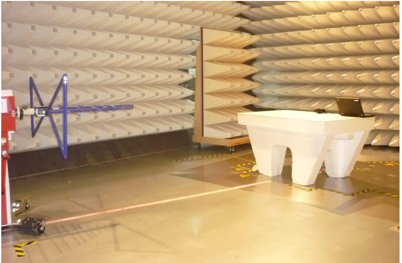
Tested frequency range 30 MHz - 1000 MHz
