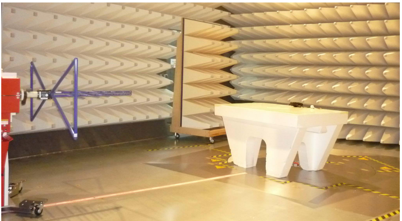
tested frequency range 30 MHz – 1000 MHz radiated
