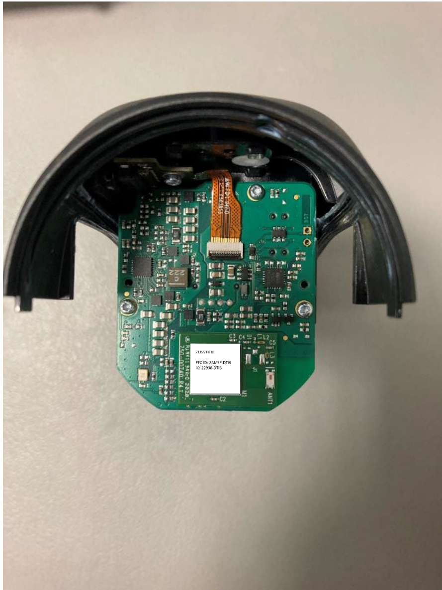
Top part with “Charge PCB” and Wifi module
