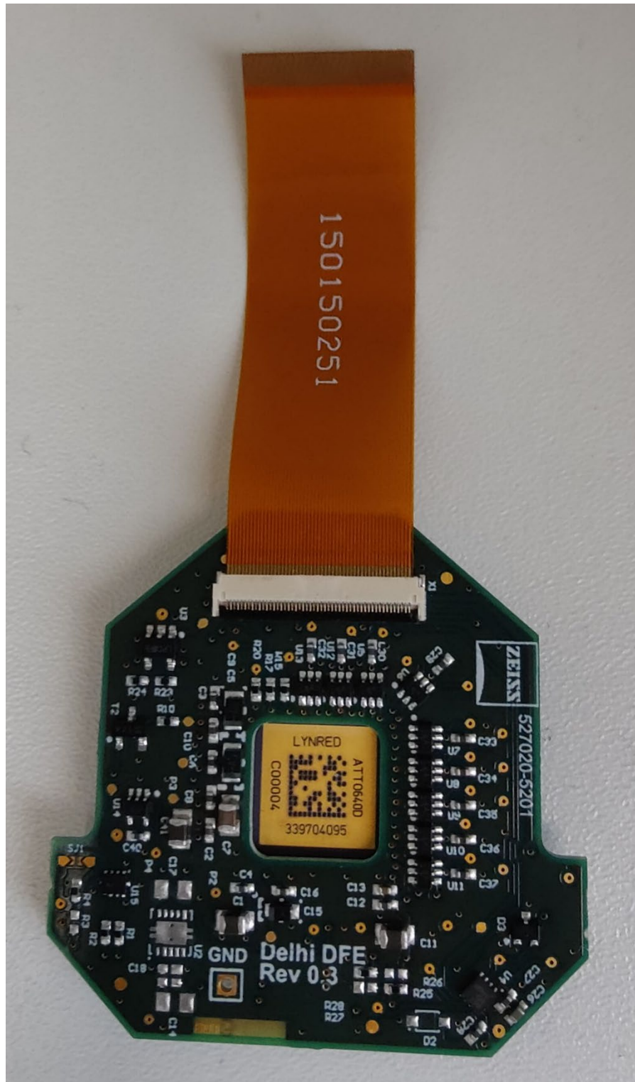
DFE Board (digital front end PCB) with infrared sensor
