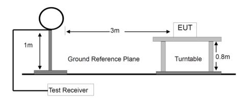
For Radiated Emission 30-1000MHz
