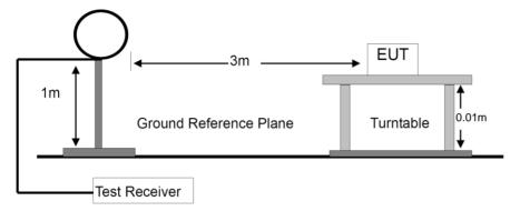
For Radiated Emission 30-1000MHz
