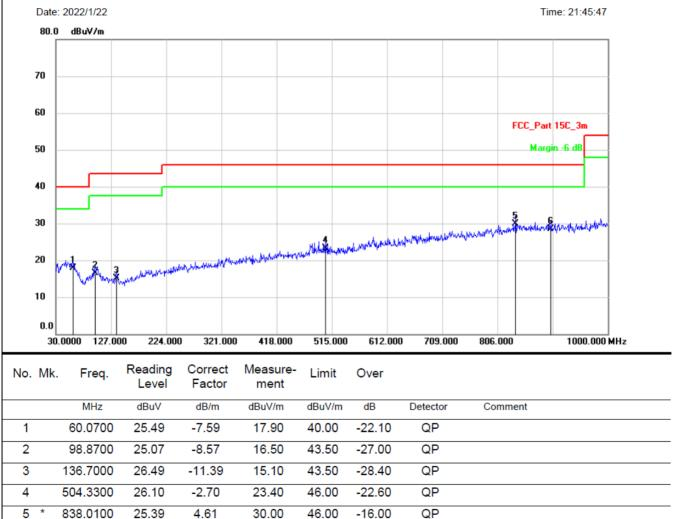
Note: Below 30MHz, the emissions are lower than 20dB below the allowable limit.
