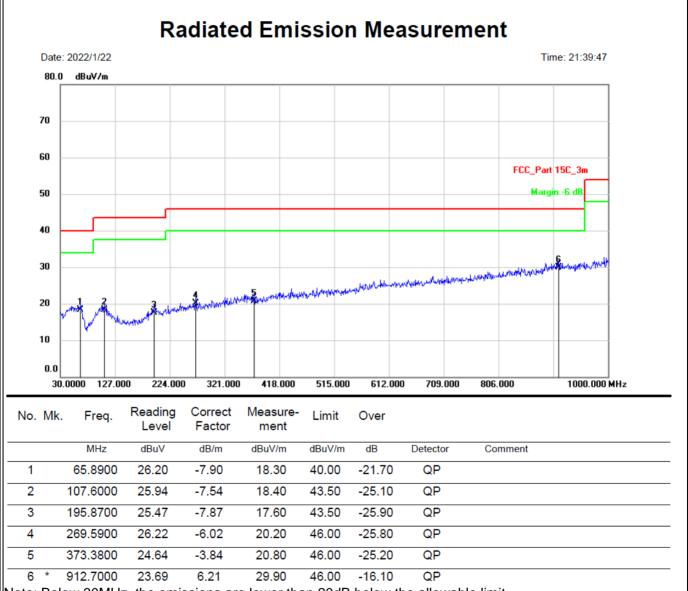
Note: Below 30MHz, the emissions are lower than 20dB below the allowable limit.
