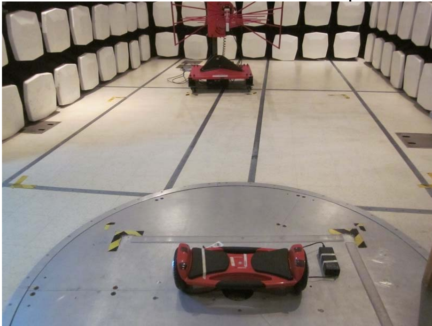
Measurement of Radiated Emission Test Set Up
