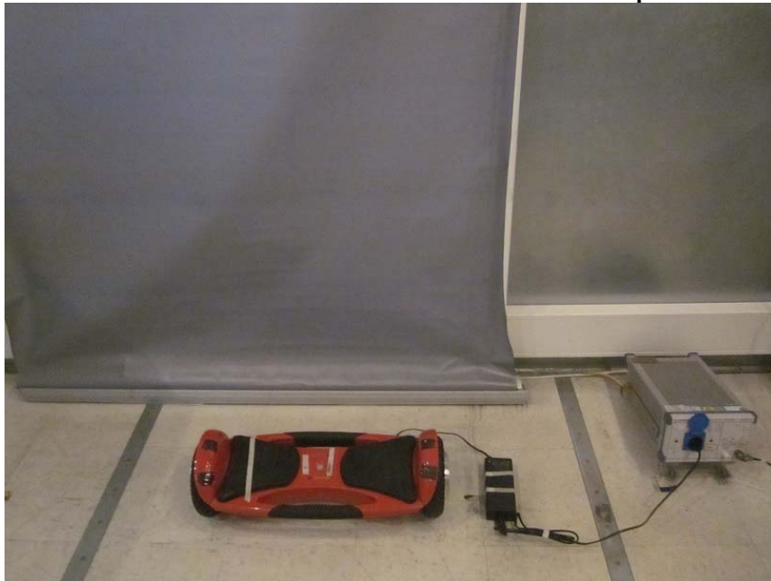
Measurement of Conducted Emission Test Set Up
