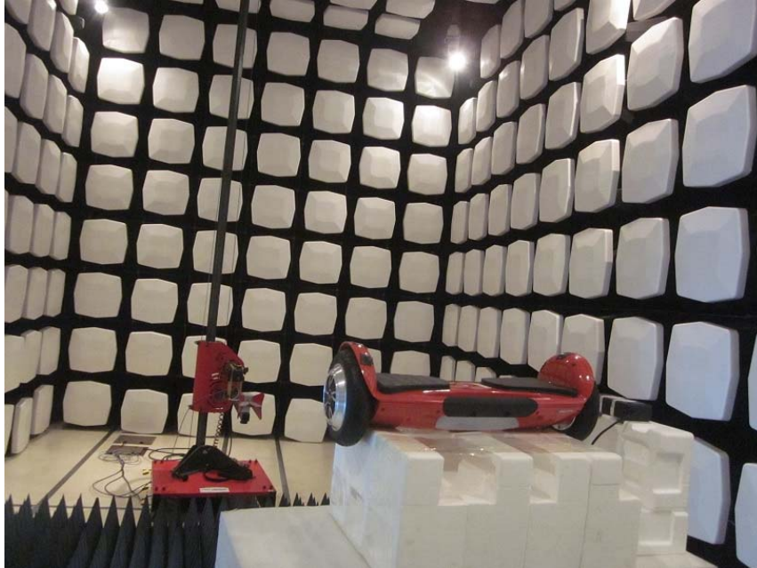
Measurement of Radiated Emission Test Set Up
