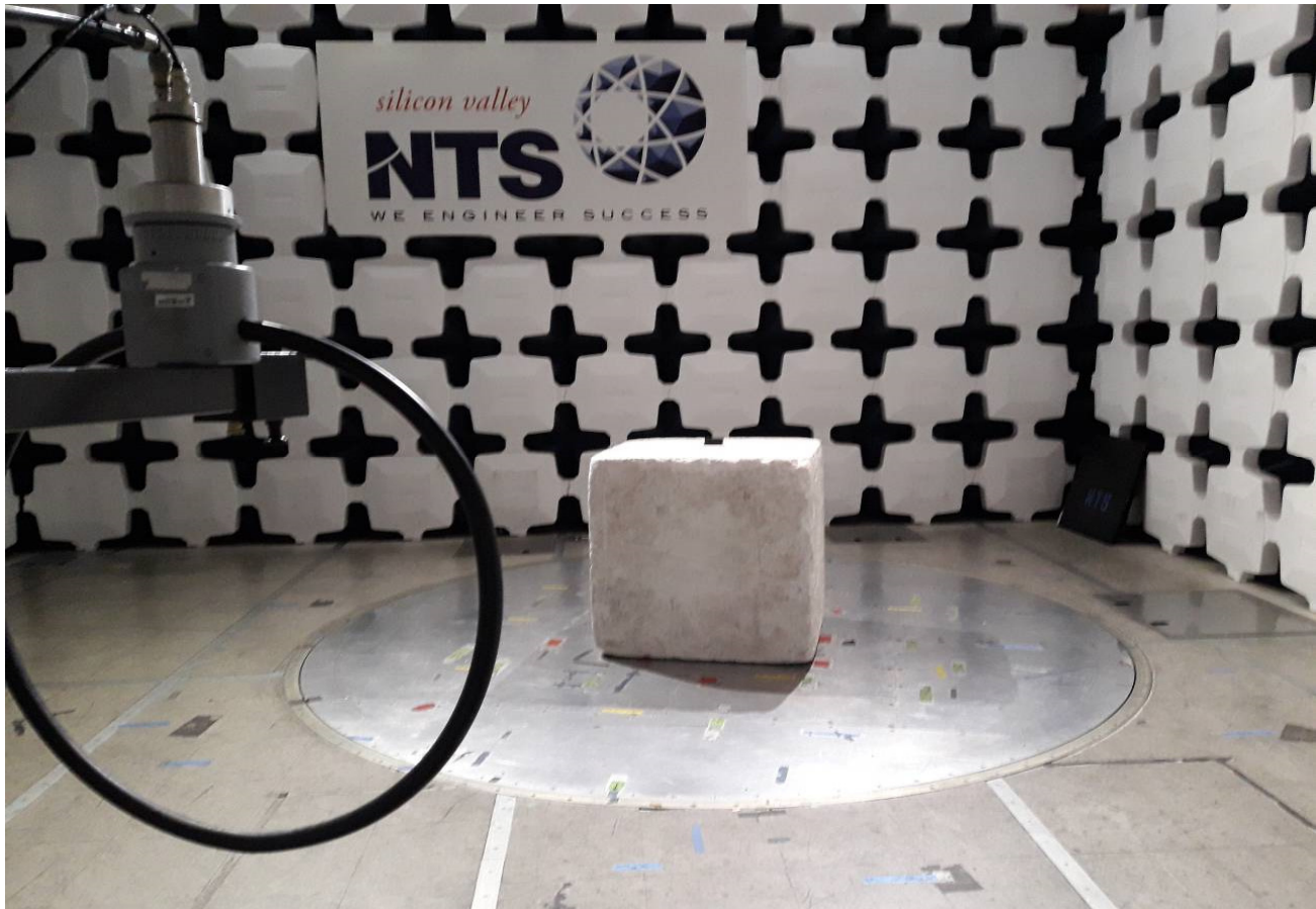
Test Configuration Photograph #1 (Radiated Emissions - Below 30 MHz)
