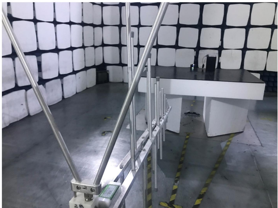
Radiation Emission Test Setup (30MHz to 1GHz)
