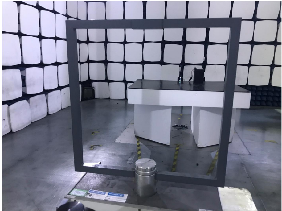
Radiation Emission Test Setup (Below 30MHz)
