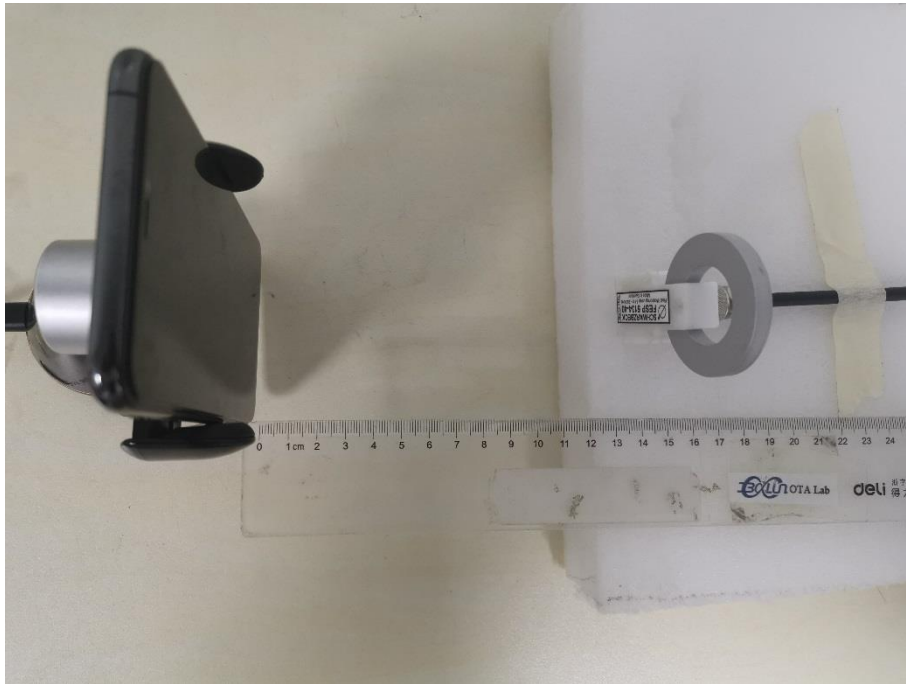
H-field Test Setup Photo Positon E (15cm)
