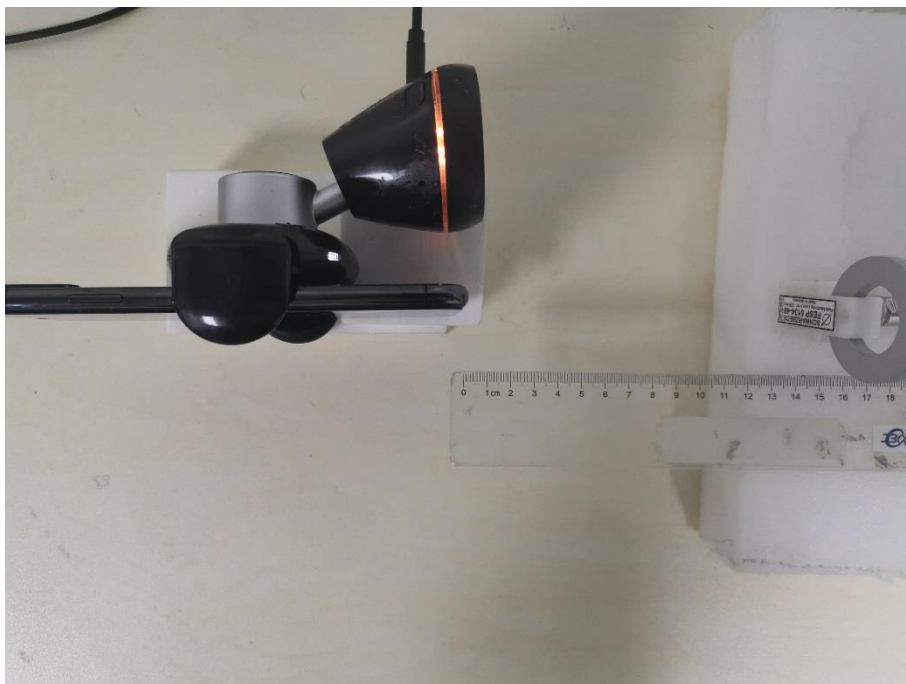
H-field Test Setup Photo Positon D (15cm)
