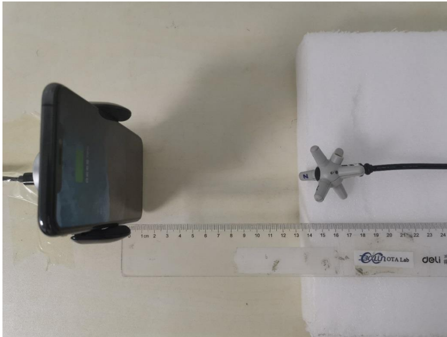
E-field Test Setup Photo Positon E (15cm)
