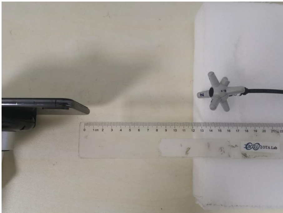
E-field Test Setup Photo Positon B (15cm)
