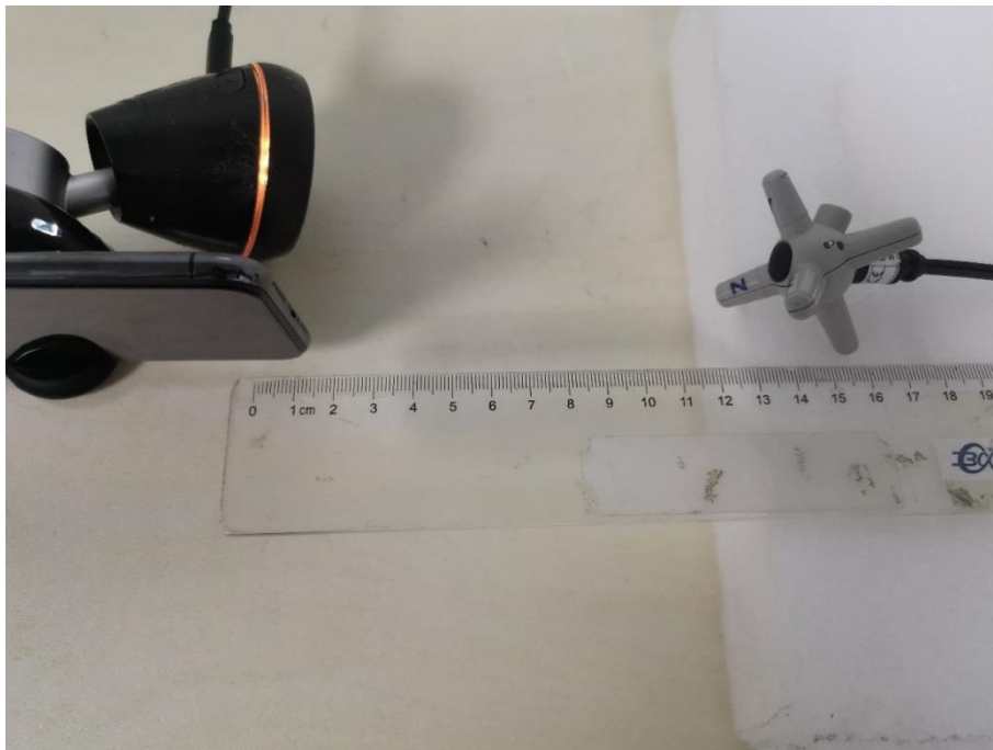
E-field Test Setup Photo Positon D (15cm)
