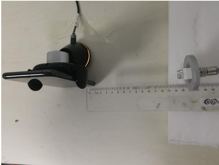
H-field Test Setup Photo Positon A (15cm)
