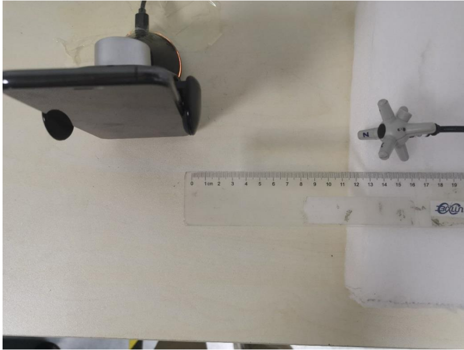
E-field Test Setup Photo Positon A (15cm)
