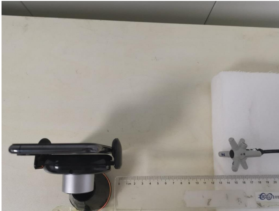
E-field Test Setup Photo Positon C (15cm)
