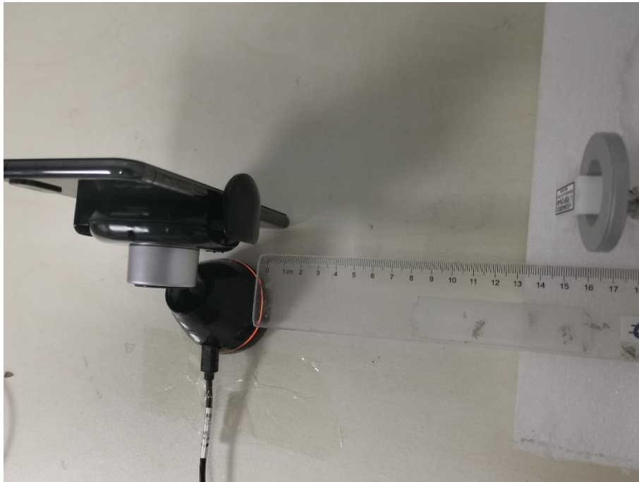
H-field Test Setup Photo Positon C (15cm)
