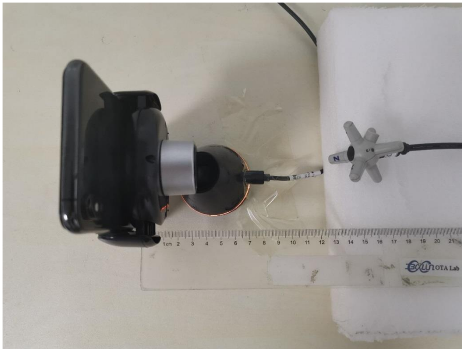
E-field Test Setup Photo Positon F (15cm)
