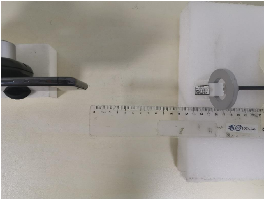
H-field Test Setup Photo Positon B (15cm)
