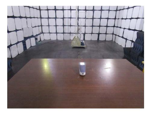
Radiation Emission Test Setup (Above 1GHz)
