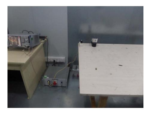
Radiation Emission Test Setup (Below 30MHz)
