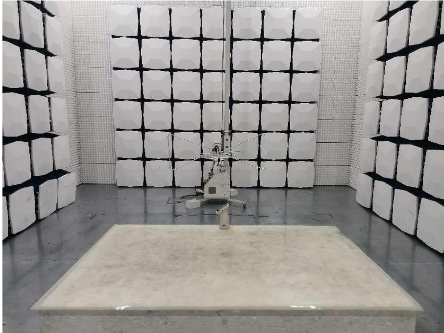
RADIATED EMISSION MEASUREMENT (below 1G)
