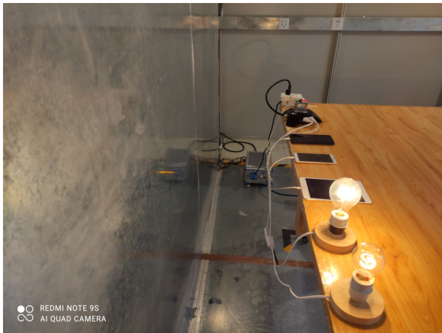
Conducted Emissions (Side View)
