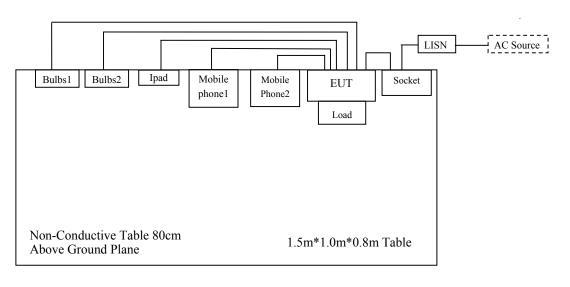
For Radiated Emissions(Below & Above 30MHz):
