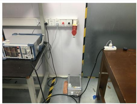
Conducted Emissions at AC Power Line (150kHz-30MHz)
