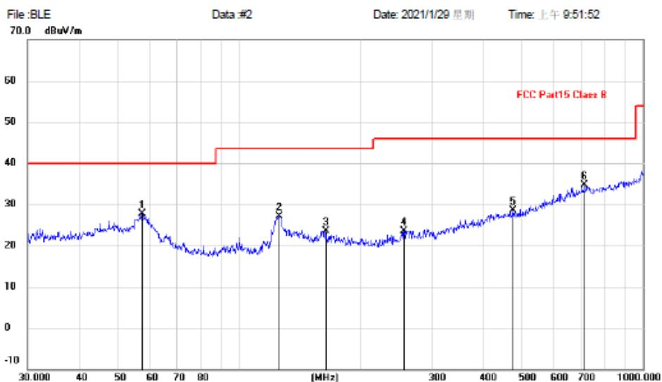
Site: FCC Part15 Class B Polarization: **Vertical** Temperature:
