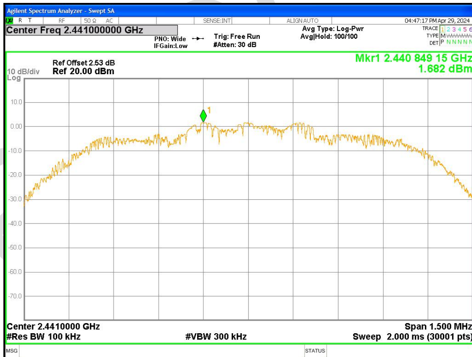
Tx. Spurious NVNT 3-DH1 2441MHz Ant1 Emission
