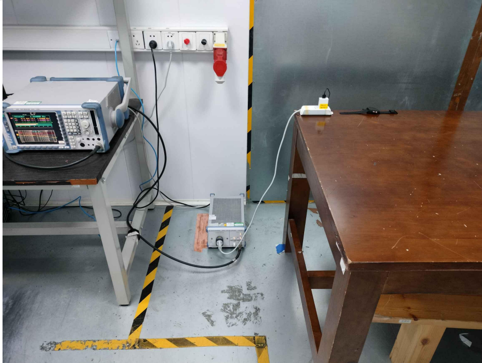
Conducted emissions at AC power line (150kHz-30MHz)
