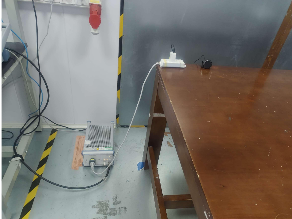
Conducted emissions at AC power line (150kHz-30MHz)
