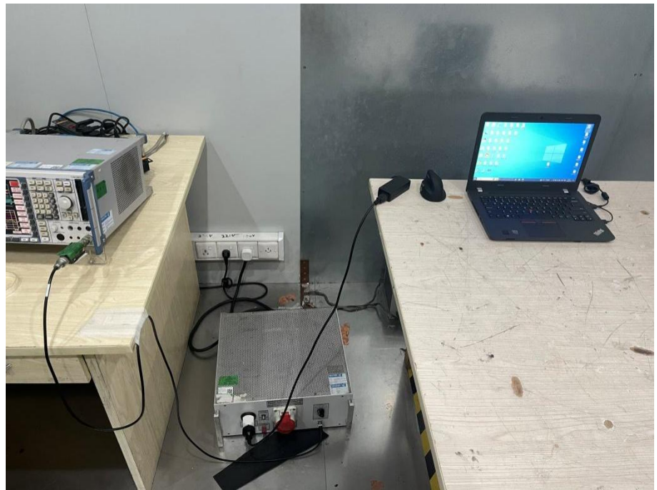
Conducted Emission Test Setup
