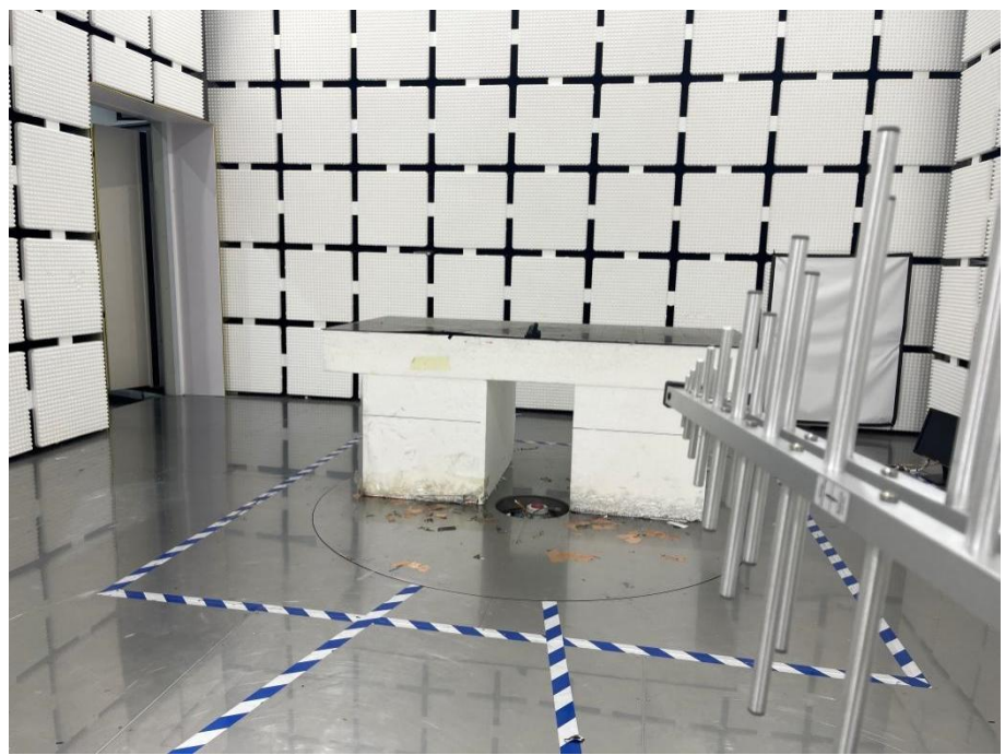
Radiation Emission Test Setup (30MHz to 1GHz)
