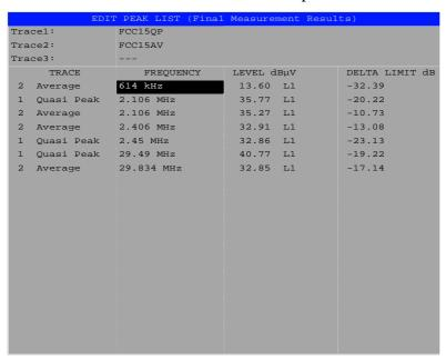
Tested Wire: Neutral Operation Mode: transmitting mode
