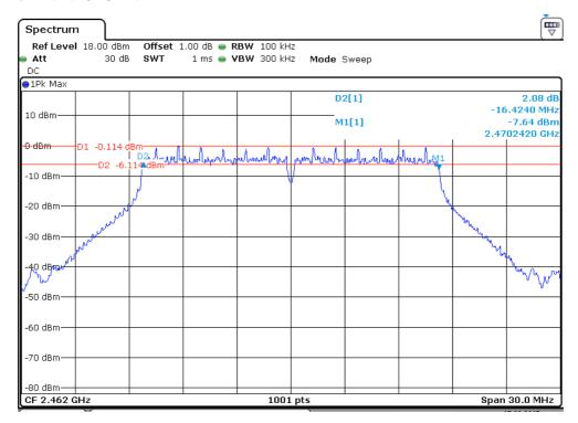
802.11n(HT20) mode with 72.2Mbps data rate Channel 1: 2.412GHz:
