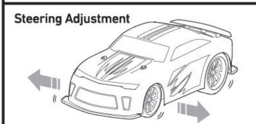
If the vehicle does not drive straight, use the adjustment dial between the front wheels.
