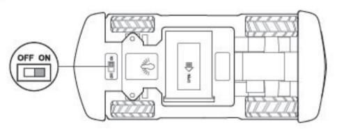
Turn the remote ON. The Pairing/Power Indicator light on the remote will flash until it pairs up with the Racer. Once paired, the light will turn off. It
